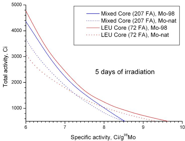
FIG. 2. Potential to produce <sup>99</sup>Mo for the mixed and LEU cores.
