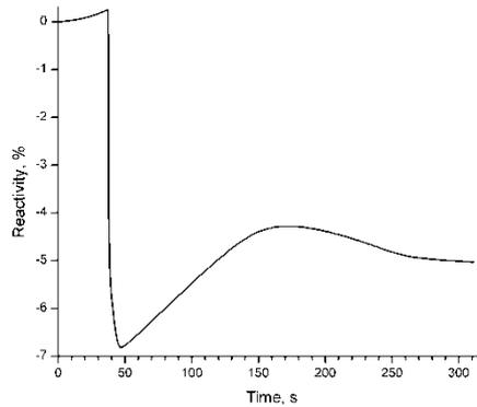
FIG. 9. Reactivity for spontaneous withdrawal of a control rod group.
