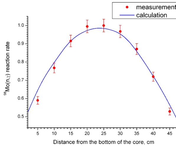
FIG. 5. Axial distribution of <sup>98</sup>Mo(n,γ) reaction rate.
