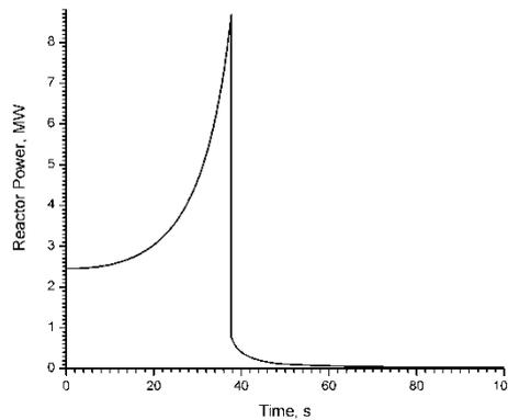
FIG. 10. Reactor power for spontaneous withdrawal of a control rod group
