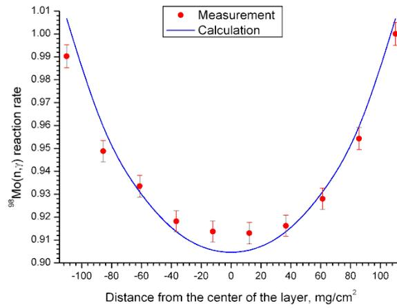
FIG. 4. Distribution of <sup>98</sup>Mo(n,γ) reaction rate through the natural molybdenum layer.
