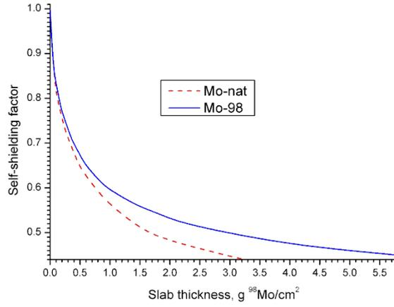
FIG. 3. <sup>98</sup>Mo(n,γ) self-shielding factor for infinite slab.
